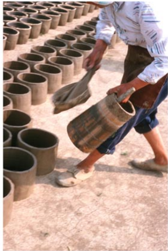
Removing mold form
